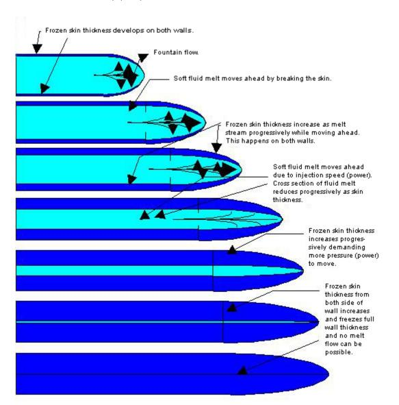
• Melt streams should reach all the boundaries of mould before melt freezes.
