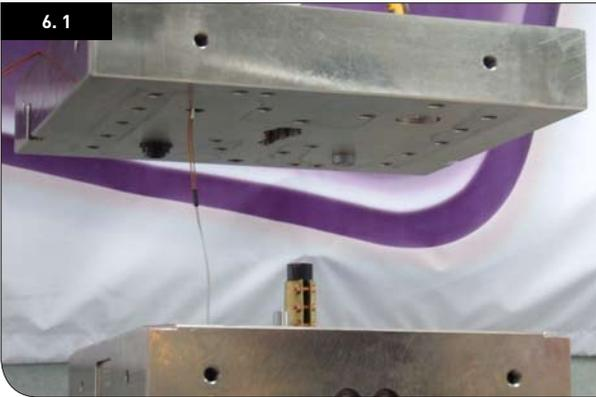
**Lower back plate onto the manifold housing plate**
