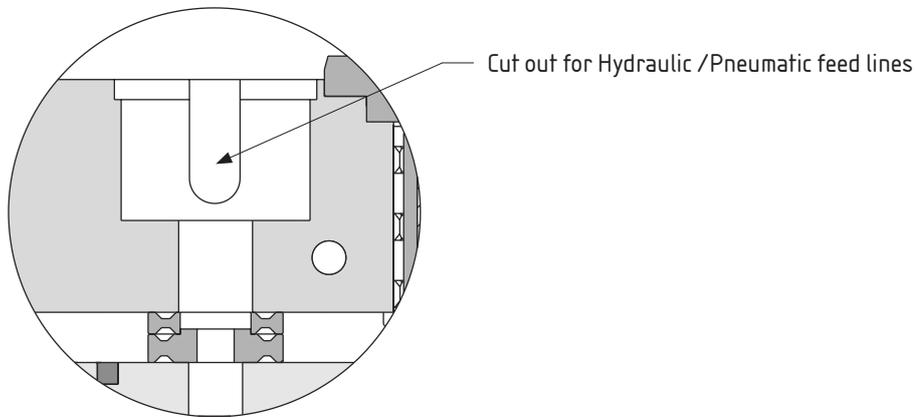
**Figure 2: Slots for Feed Lines**
