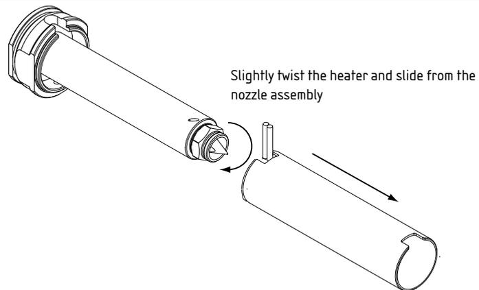
Figure 71: Remove Heater from an MX nozzle
