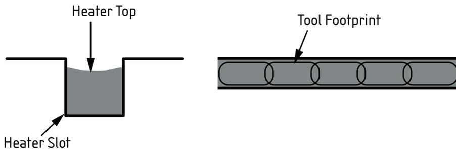
Figure 53: Pressed-in Heater Top after Correct Installation
