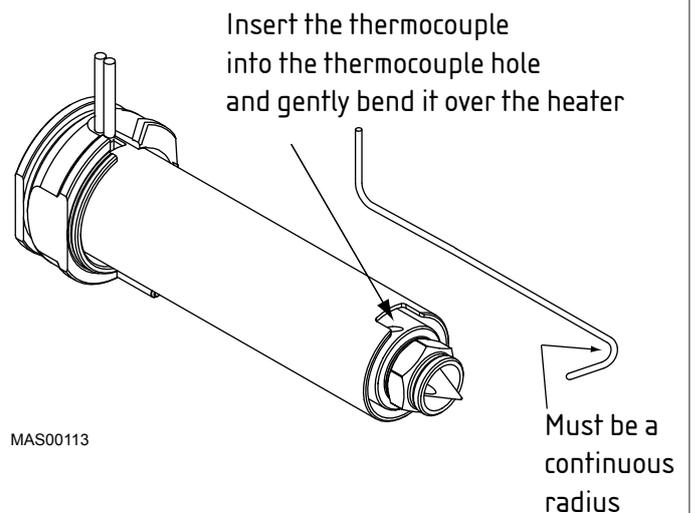
Figure 34: Insert Thermocouple on MX Nozzle
