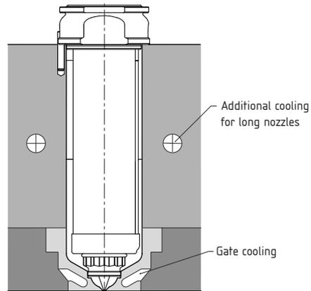
Figure 14: Insert with Cooling Channel Groove Example
