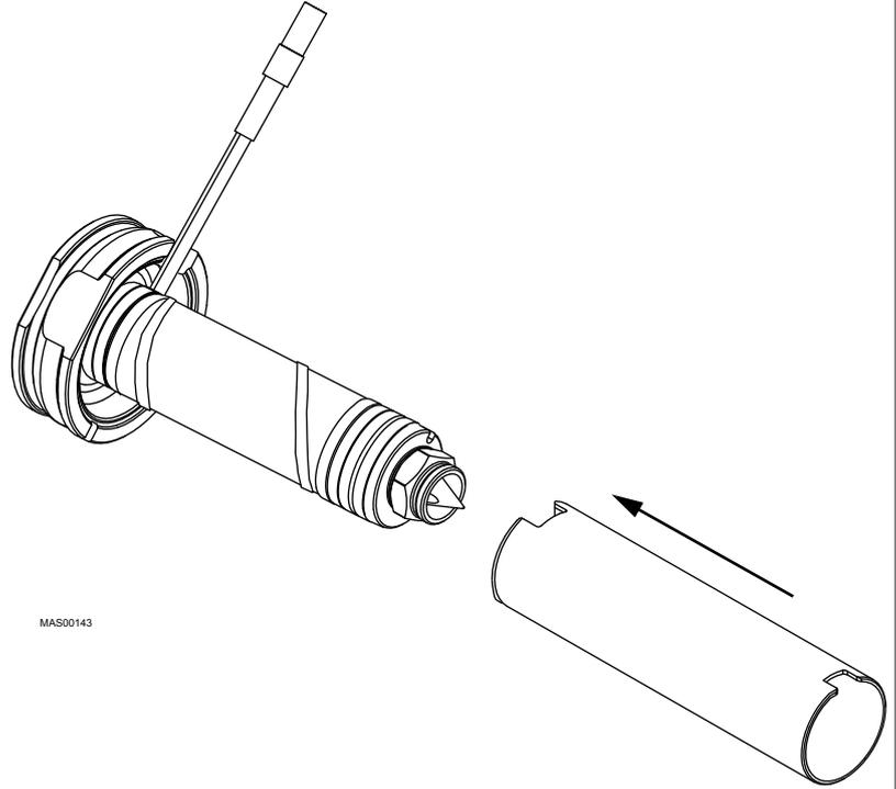
Figure 79: Slide on BX or SX Heater Cover
