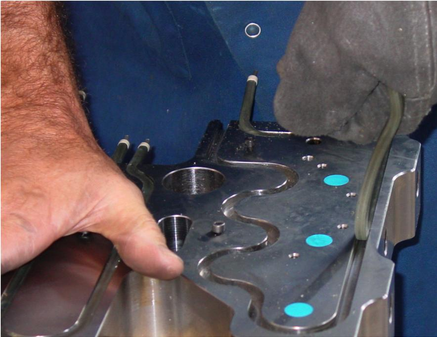
**Figure 49: Pull Pressed-in Heaters out of Straight Sections**
