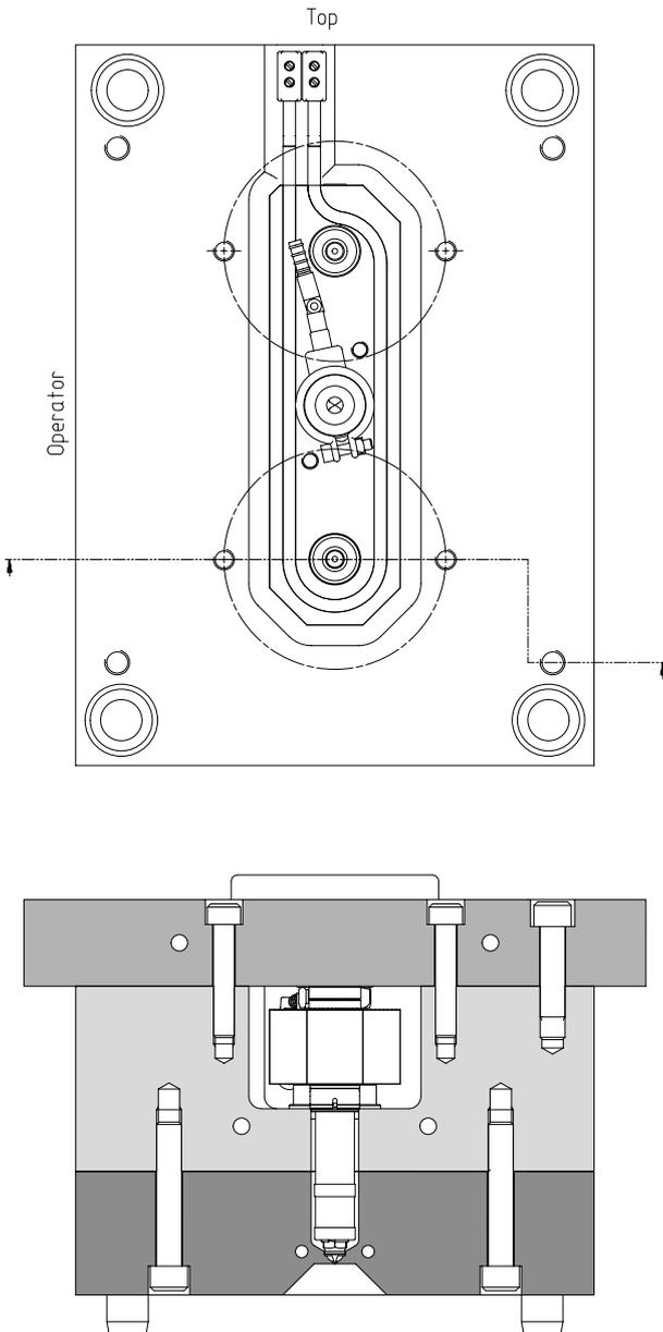
**Figure 12: Suggested Placement of Clamping Bolts**
