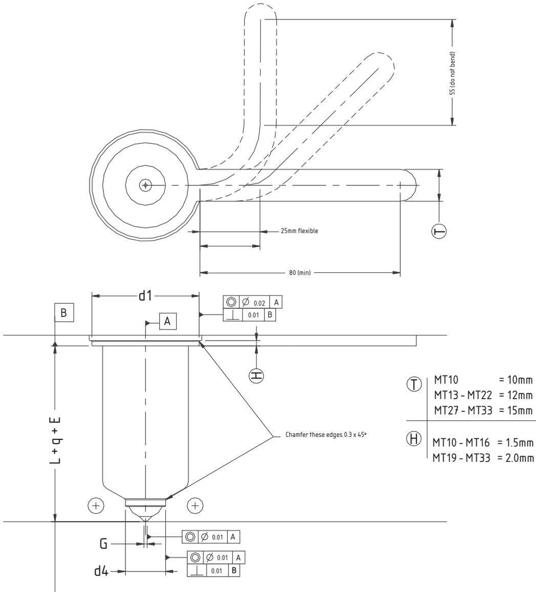
**Figure 19: MT Range Nozzle Installation Tolerances**
