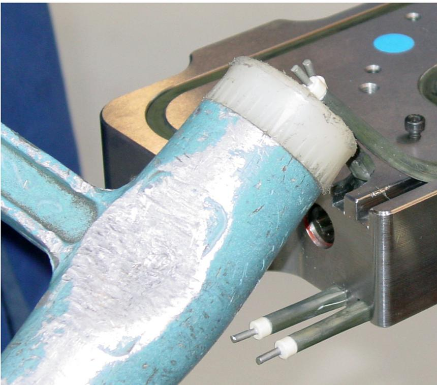
**Figure 46: Using a Hammer to Bend Up the Ends of a Pressed-in Heater**
