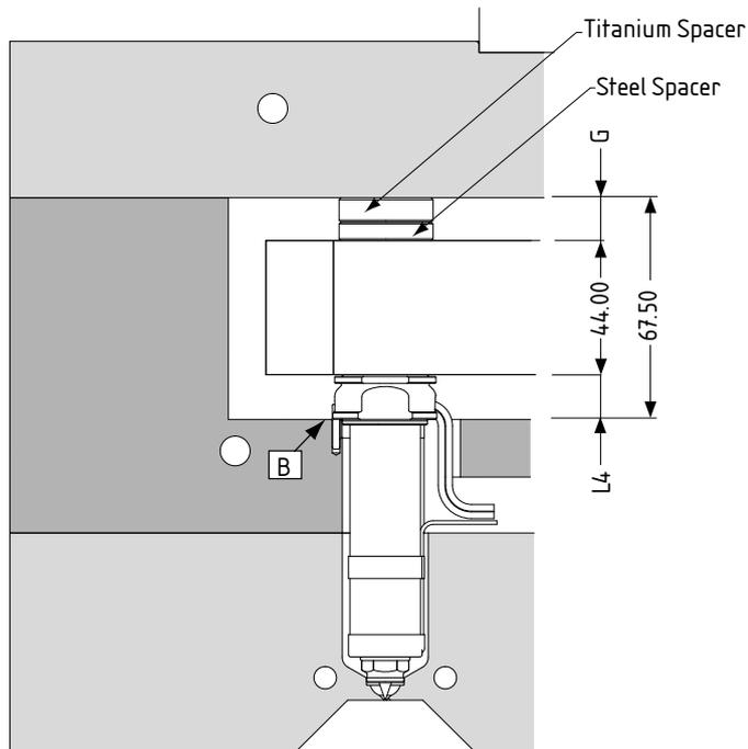
Figure 6: Measurements Needed for Manifold Expansion Calculation (Thermal Gate)
