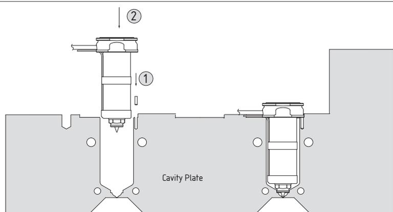
Figure 20: Insert BX Nozzles
