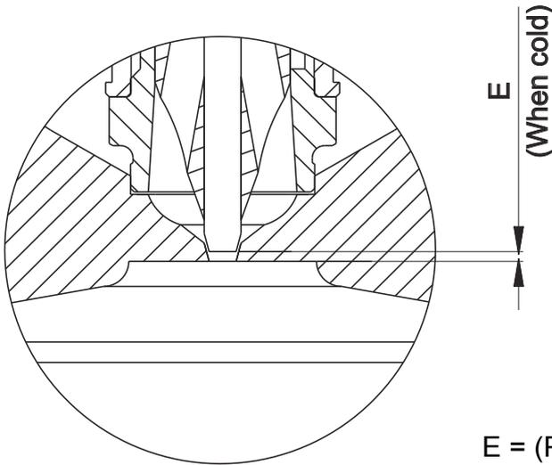
$$E = (\text{Pin Length} - 25) \times k \times \Delta \text{Temp.}$$
