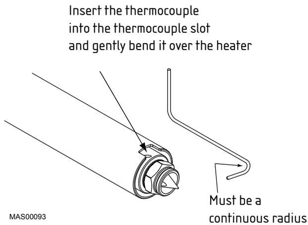
Figure 27: Install Thermocouple on MX Nozzle
