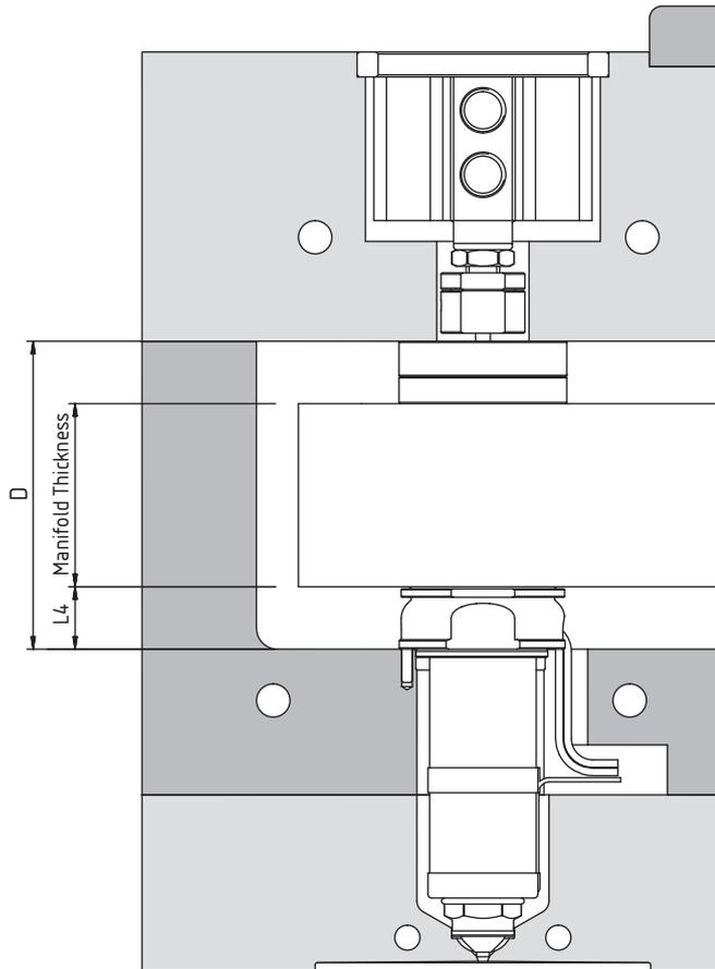
**Figure 7: Measurements Needed for Manifold Expansion Calculation (Valve Gate)**
