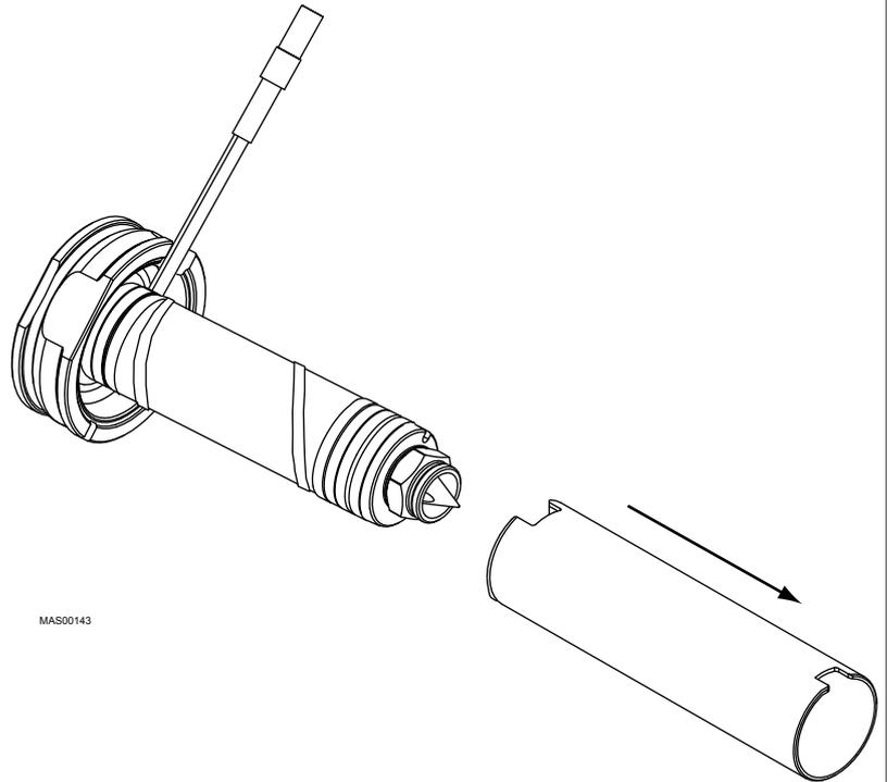
Figure 77: Slide off BX or SX Nozzle Heater Cover
