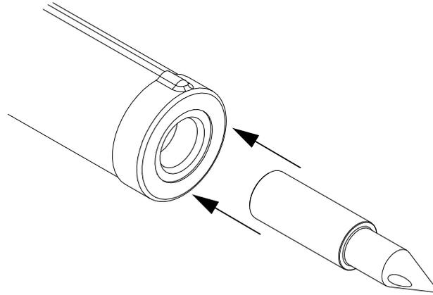
Figure 63: Insert Tip in an X Range Nozzle
