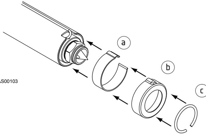
Figure 32: Finish MX Nozzle Installation
