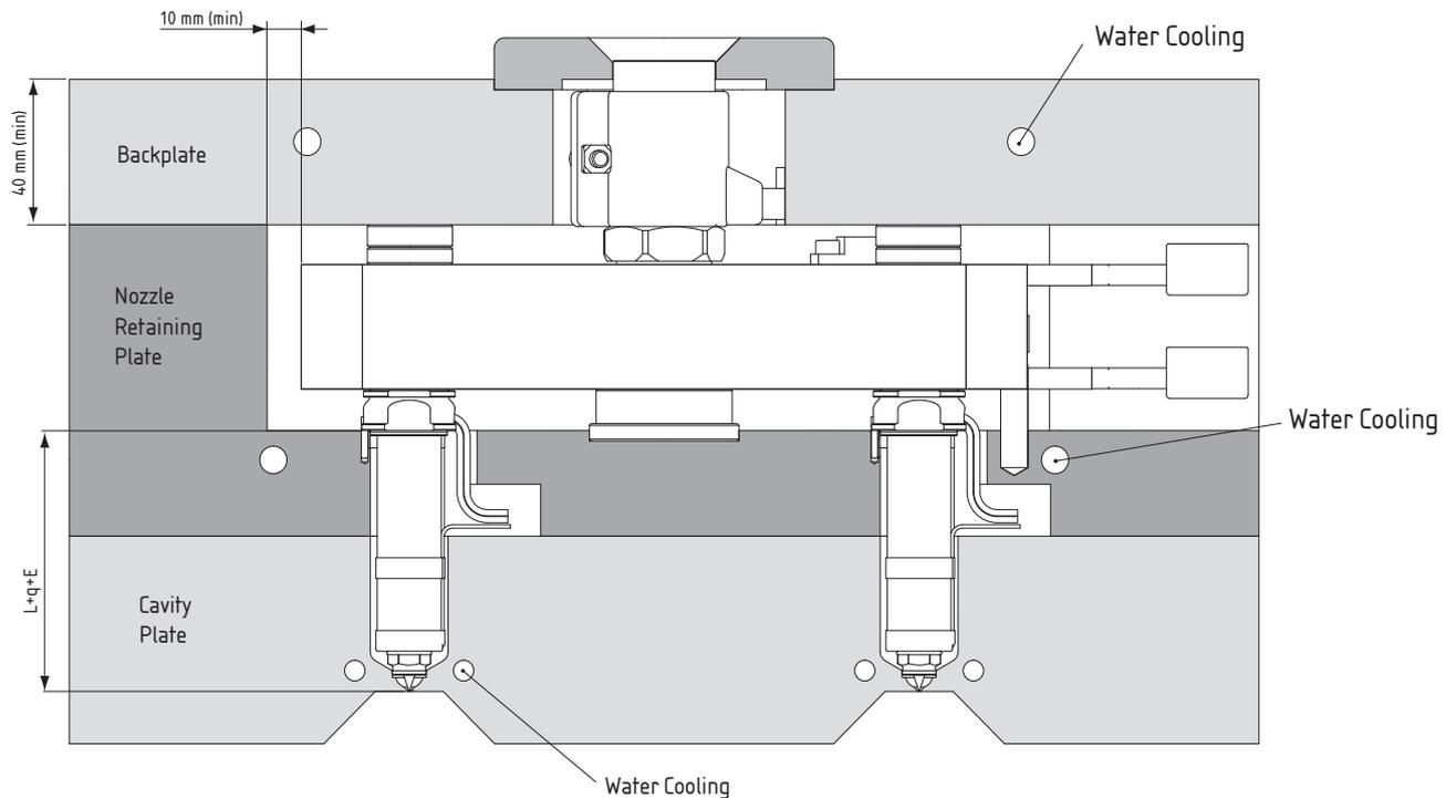
**Figure 1: Example Layout for a High Production Manifold**
