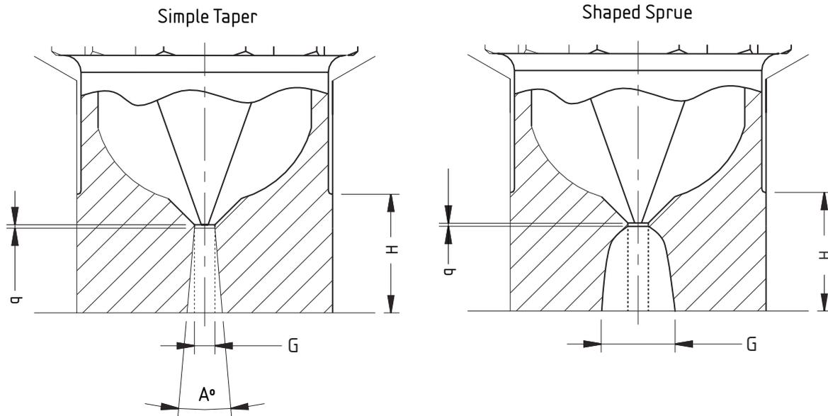
**Figure 4: Sprue Nut Gate Land Modification Examples**
