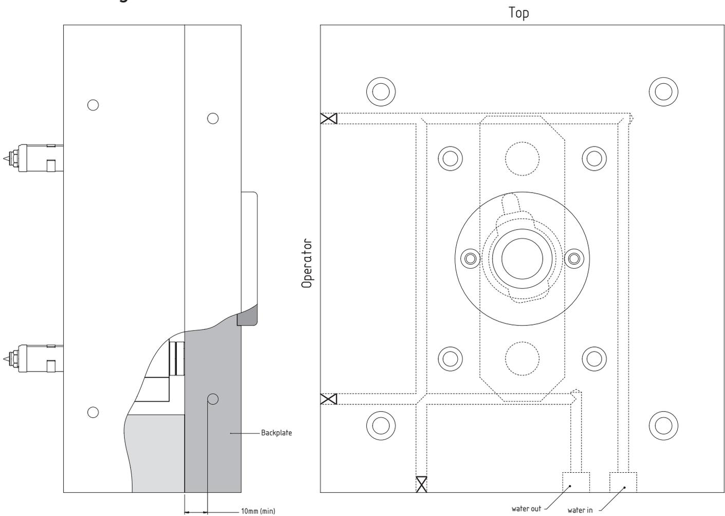
**Figure 16: Typical Cooling Channels in the Back Plate of the Tool**
