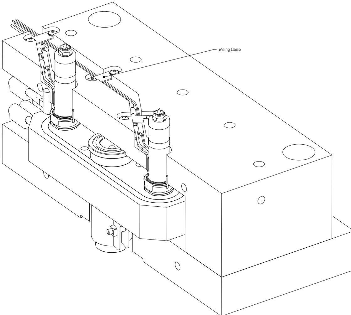
**Figure 17: Manifold Wiring Diagram (Cutaway view)**
