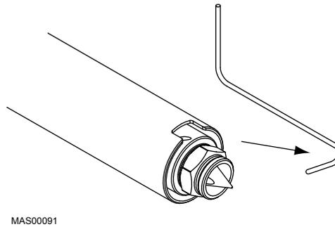
Figure 76: Remove Thermocouple from a BX or SX Nozzle
