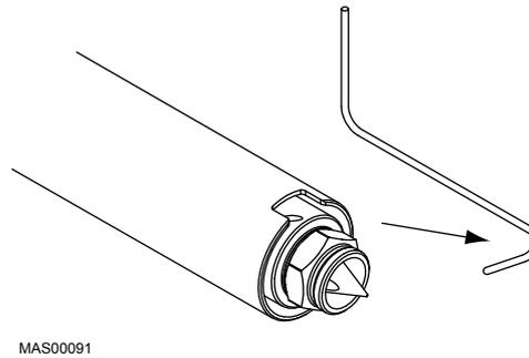
Figure 70: Remove Thermocouple from an MX Nozzle
