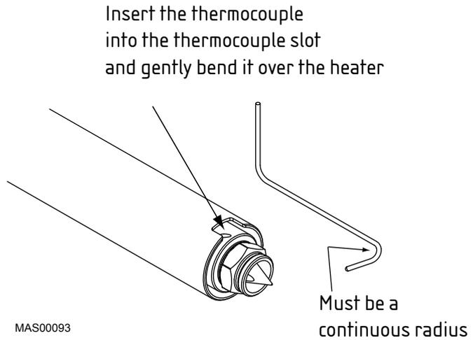
Figure 67: Install Thermocouple on an X Range Nozzle
